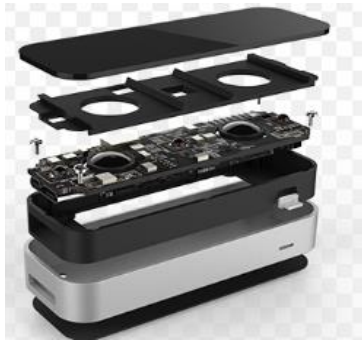
Fig. 2 Inner Parts of Leap Motion Controller
