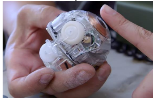
Fig. 8 Inside structure of a BB 8 sphero toy
